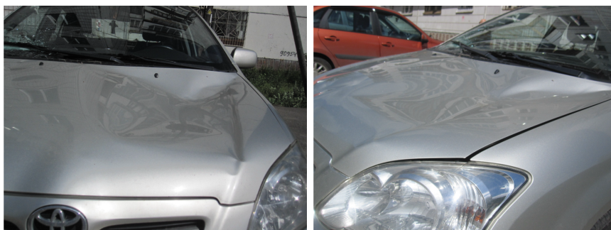
Fig. 5. Photos of the car damaged as result of falling of snow heap
